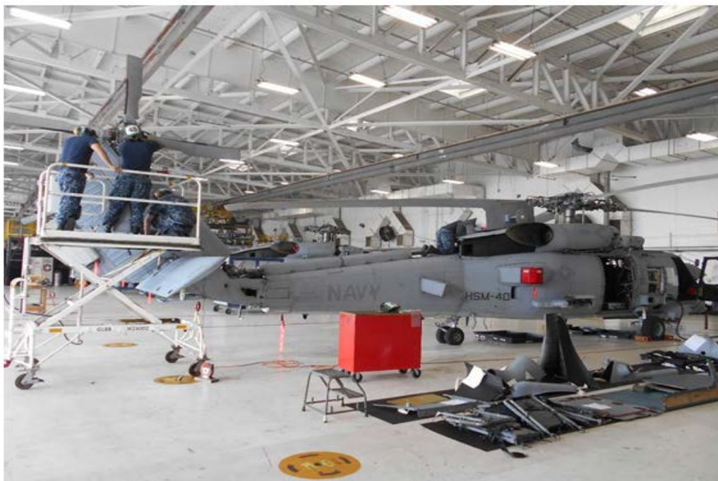
Figure 4. B-4 stand with swing gate taped open and no end rails used for access to the tail rotor. Work on top of the aircraft with no fall protection aft of the main rotor can also be seen.
